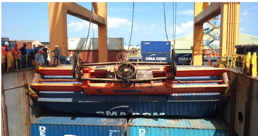
**June 28, 2010: Port of Longoni:** While lifting the container, the stacker tilted over damaging the container beyond repair. Stacker operator was not seriously injured due to cabin safety belt. Declared cargo gross weight was 16,890 kilograms. Actual gross weight as established by the harbor weighing bridge after the incident was 30,220 kilograms.
